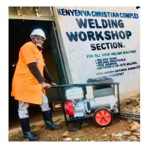
Since a welding machine requires electricity, the ability to make products and repair broken metal objects was severely hampered. It's not uncommon for the power to be out three days a week. The answer to that problem is to purchase a welding generator, which costs a good bit more that a standard gas-powered generator.
